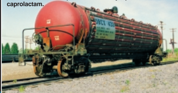
ControTrace elements on this rail car solved a critical maintenance problem for a major producer of caprolactam.
